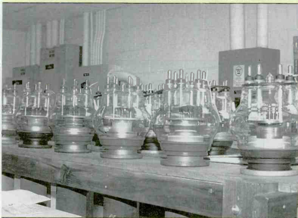
Power transmitter tubes are driven hard enough for their plates to glow red. Several spares are kept on hand.
