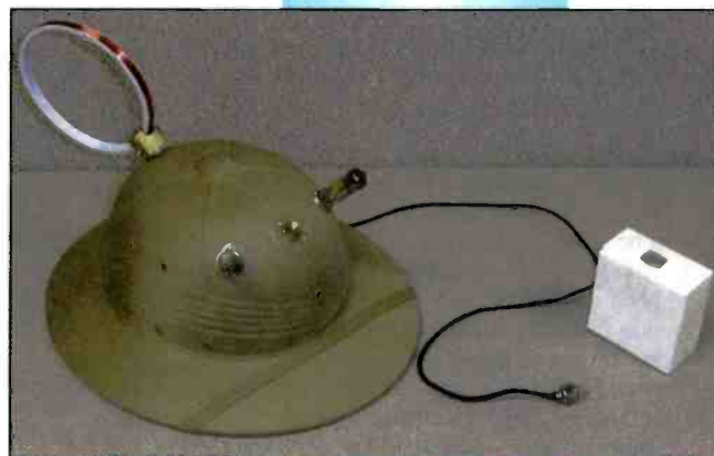
The hat is tuned using a tuning capacitor and knob recycled from a junked transistor radio. Note the loop antenna assembly; Bill uses a quarter-inch phone plug to permit tilting the loop for the best signal.
