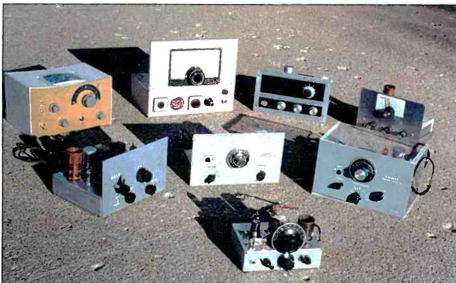
Al Cikas, KAGDL's growing family of homebrew Ocean Hoppers! This shot shows the original Allied Ocean Hopper receiver and the seven homebrew versions it inspired.
