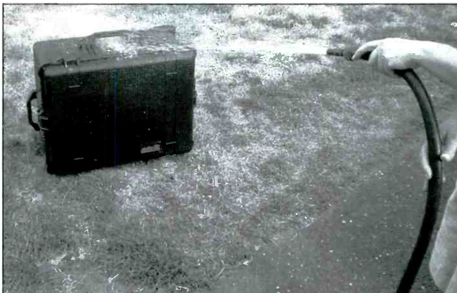
Try this with your luggage (but be sure none of your family's stuff is inside). The Pelican 1620 case kept all the radio gear dry despite this extensive drenching.
